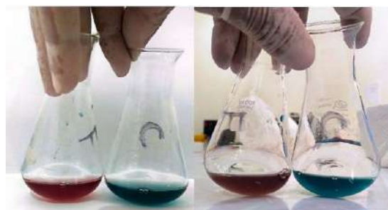
Pictorial view of screened reagents color development for detection of zinc in wheat flour samples
