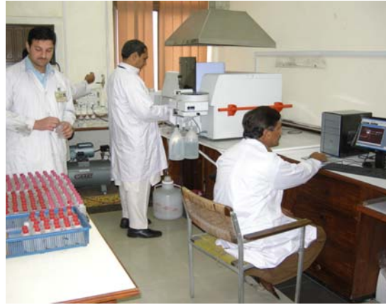
Micronutrients analysis on atomic absorption spectrophotometer in progress
